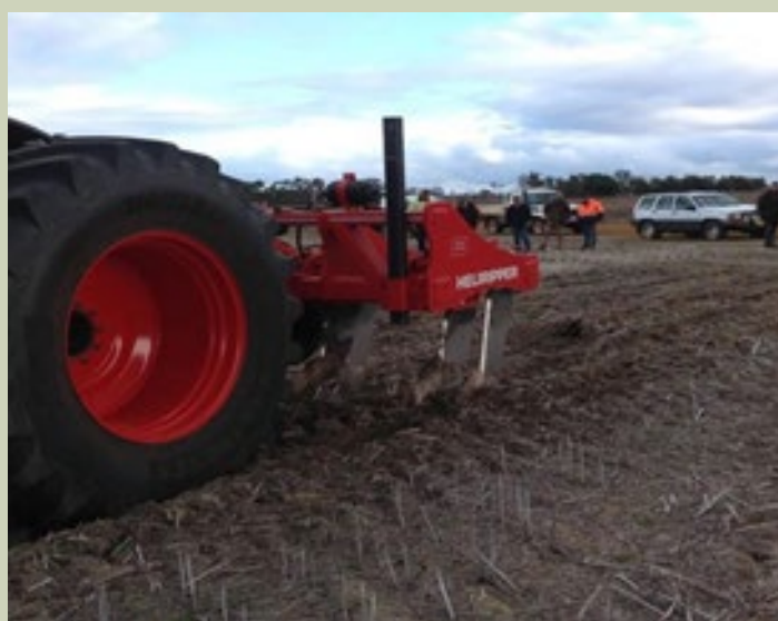
FIGURE 1: Deep ripping at Kojaneerup site with Heliripper
