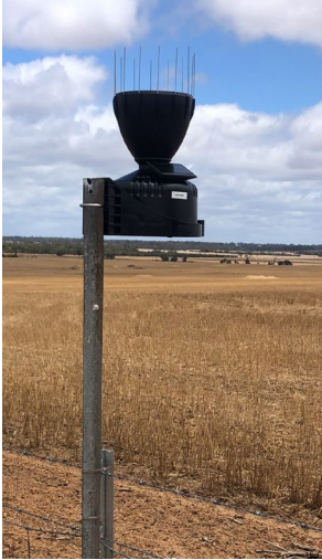
AxisTech Rain Gauge
