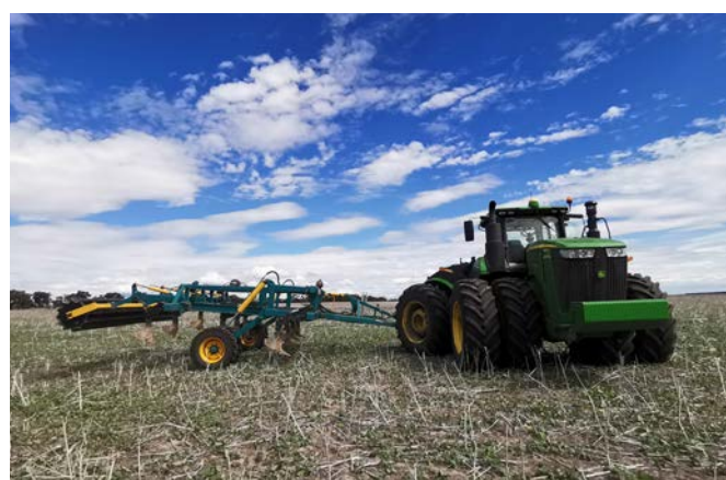
Figure 2: Image of Nufab deep ripper used to achieve an approximate 500mm deep amelioration.
