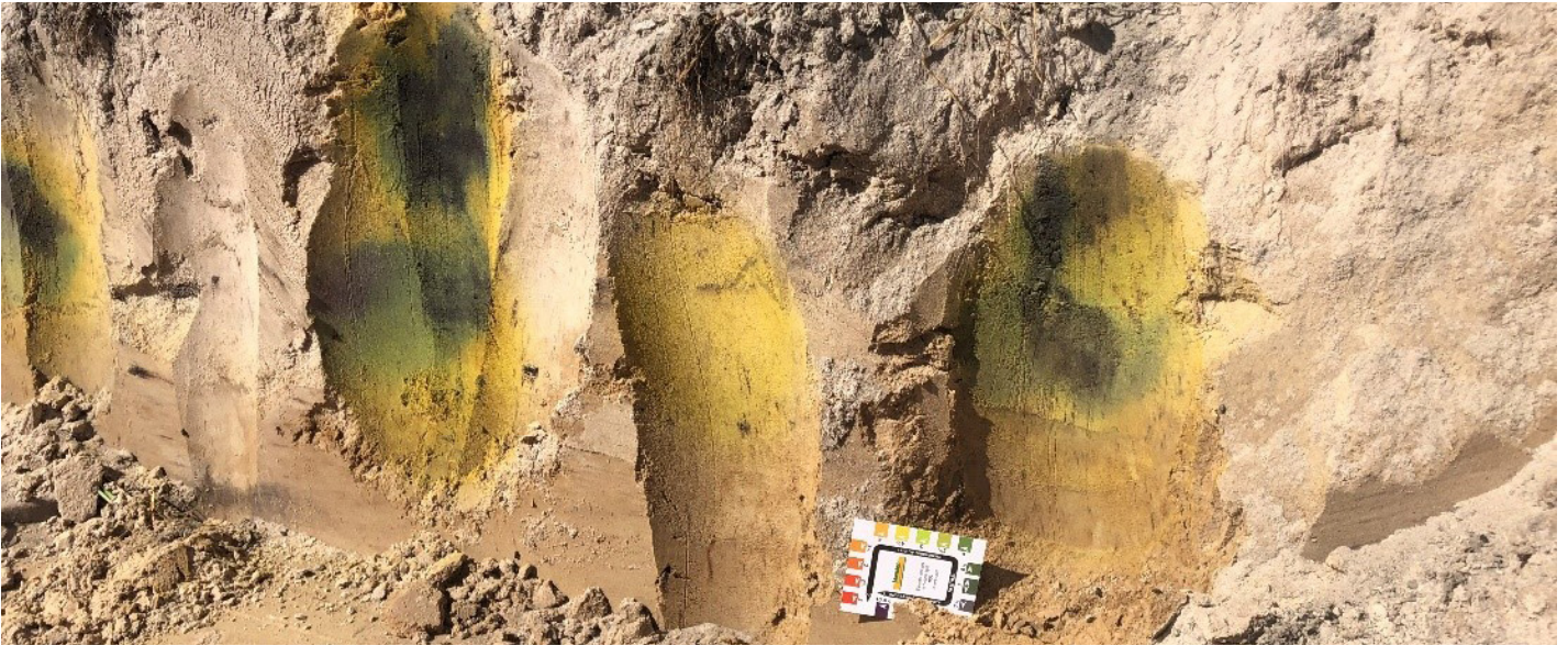
▲ Figure 2: Image of a deep rip plus lime soil pit. The purple indicator shows lime has relocated down the ripper type in the subsoil.
