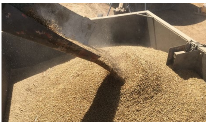
Photo 1. Barley moving from the auger into the hopper of the snail roller. A sensor ensures the hopper remains full to maximise grain turnover and improve snail removal.
