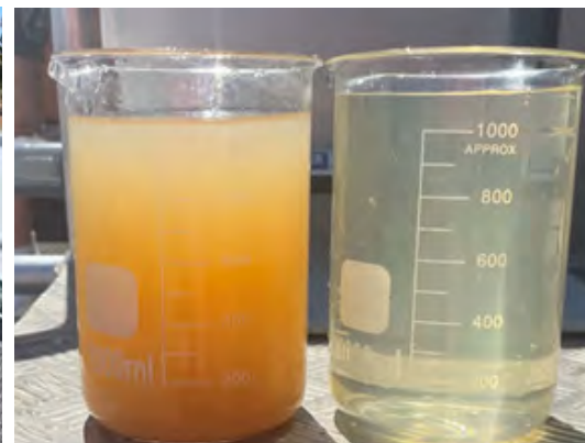
Left: The CBH tarp installed on the Jacup catchment. Middle: Checking out how the filtration system works. Right: A comparison of the dam water before and after being pumped through a ceramic filtration system
