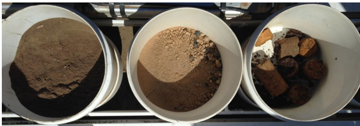
Figure 5 - Loamy Clay duplex at Central Woogenellup. Left bucket is (0-10cm), centre bucket is (10-20cm) and right bucket is (20-30cm).
