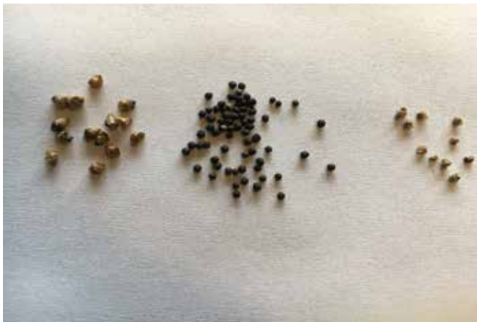
▲ Figure 2: Snails on the left were removed from the canola (centre) using a rotary grain cleaner with 2.5mm slotted screens. The snails on the right could not be removed using the same screens.
