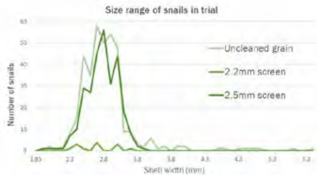
▲ Figure 1: Graph showing the size range of small conical snails found in a) uncleaned canola, b) canola cleaned with a 2.2mm slotted screen and c) canola cleaned with a 2.5mm slotted screen. Number of measurements: Uncleaned CANS = 360, 2.5mm = 282, 2.2mm = 19.
