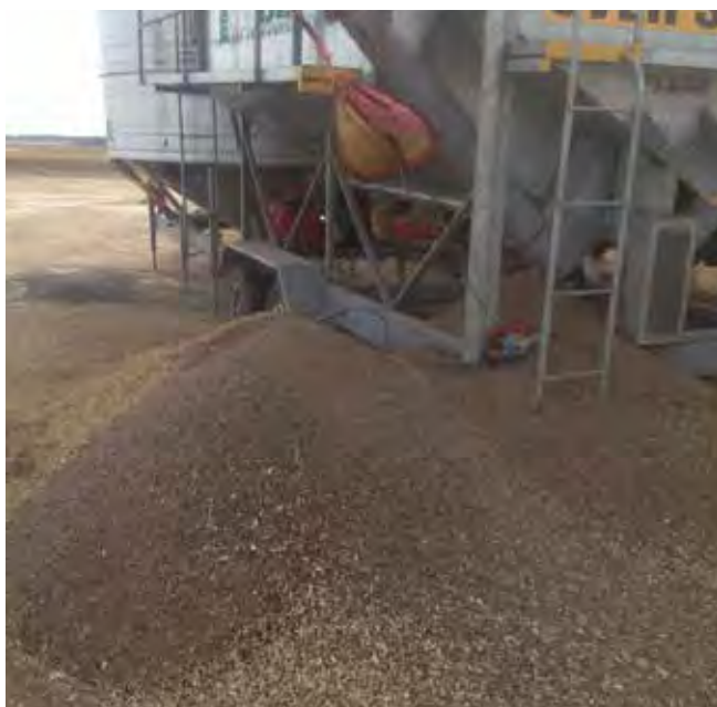
▲ Photo 1: A pile of small conical snails removed from canola using a 4-barrel rotary grain cleaner with 2.5mm slotted screens.
