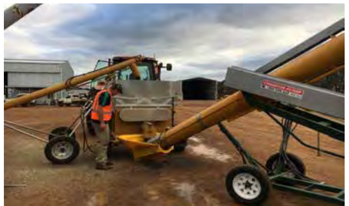
▼ Photo 3: The snail roller processing canola during the trial.
