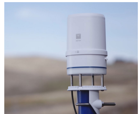
Figure 2: Atmos 41 All-in-one device. (source: Meter Group)
