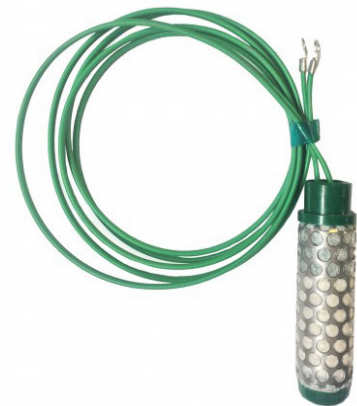
Figure 5:Watermark Soil Moisture Sensor.
