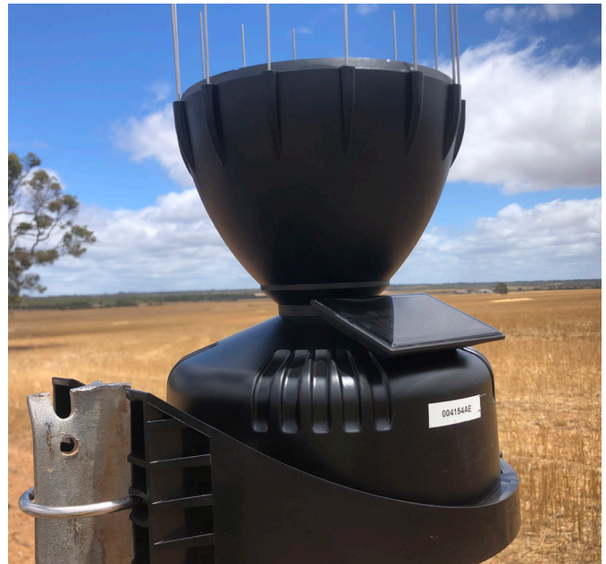
Figure 3: Sigfox connected remote rain gauge on the SCF Smart Farm.
